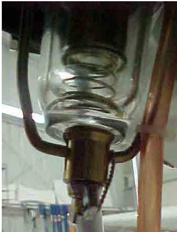
**Figure 7.65:** Fuel Filter Safety Wire
