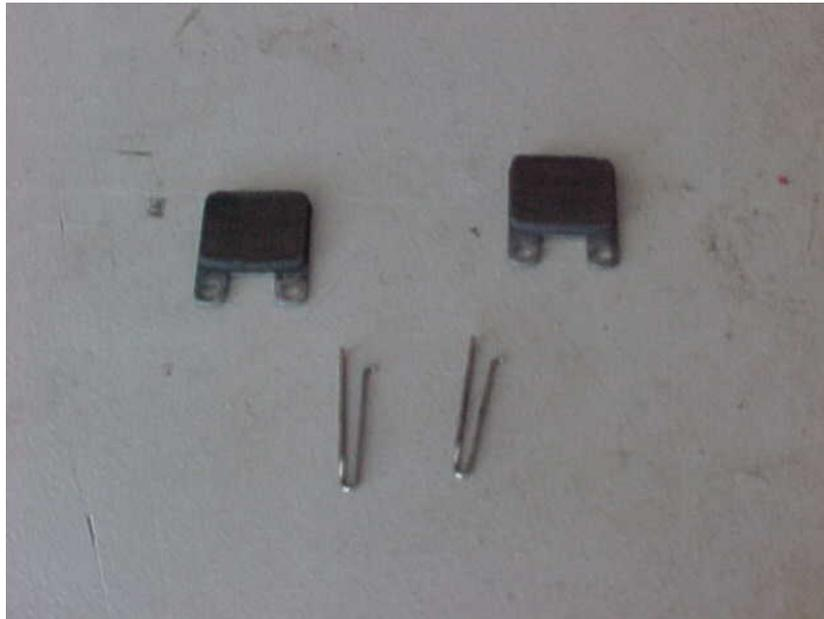
**Figure 7.6** Brake pads and retaining pins
