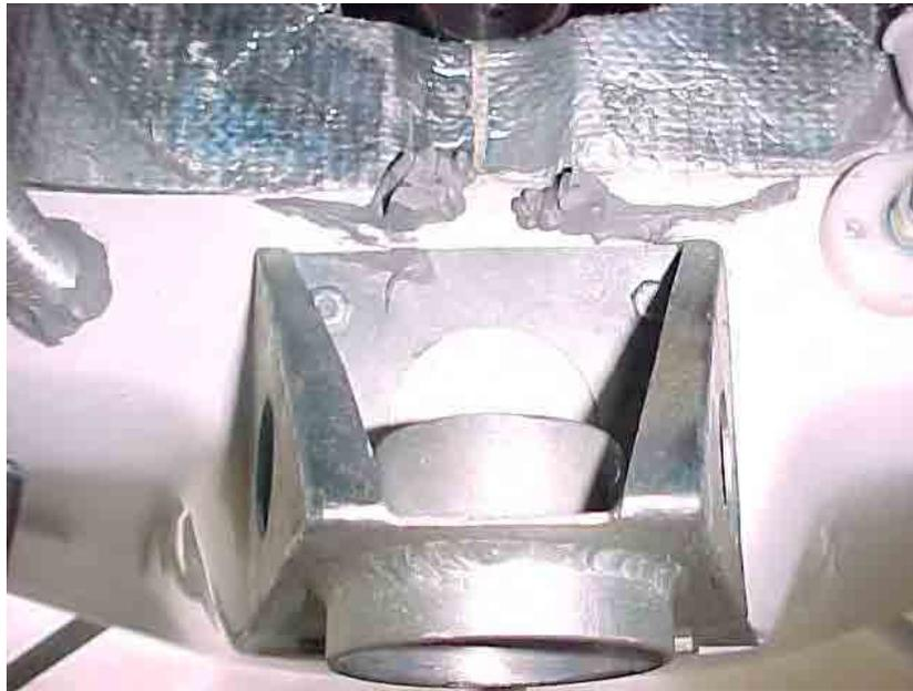
**Figure 7.39** Lower nose strut bearing housing
