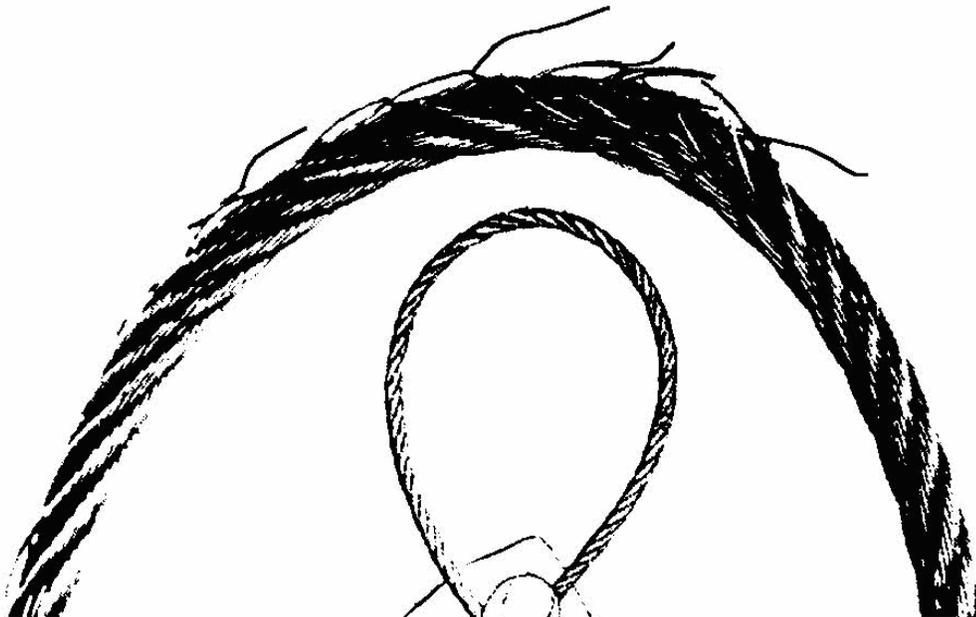
**Figure 7.77** Wire cable strands exposed by bending the cable.
