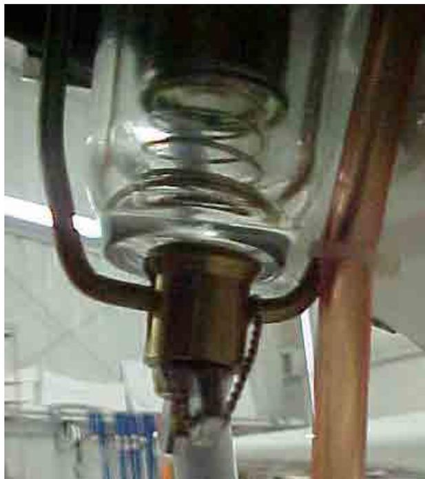
**Figure 7.68:** Fuel Filter Safety Wire
