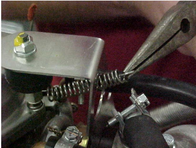
**Figure 7.49** Carb support spring removed
