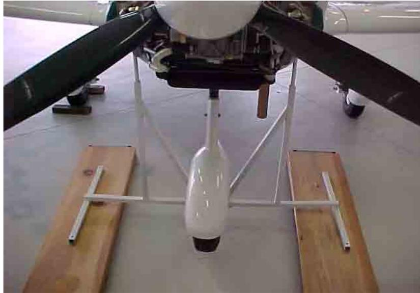
**Figure 7.27** Nose strut on supports with chocks on main gear
