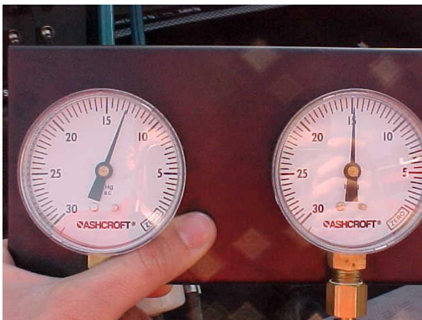
**Figure 7.58** Initial reading of imbalanced manifold pressures
