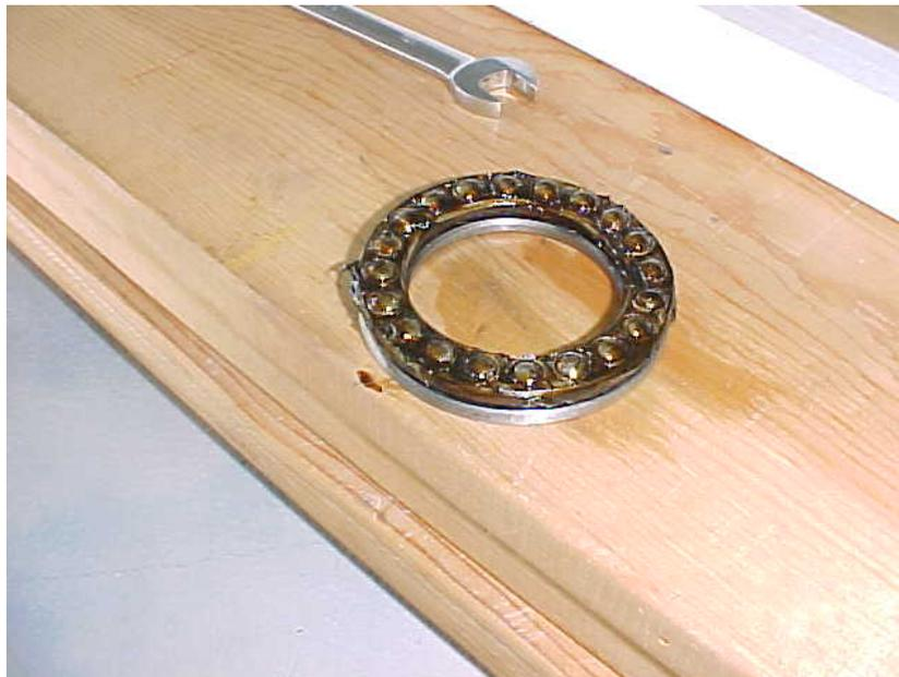
**Figure 7.36** Lower nose strut bearing and race
