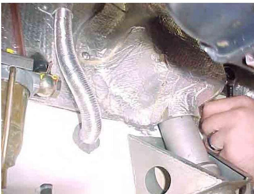
**Figure 7.43** Reseal fire resistant material around the firewall cover.
