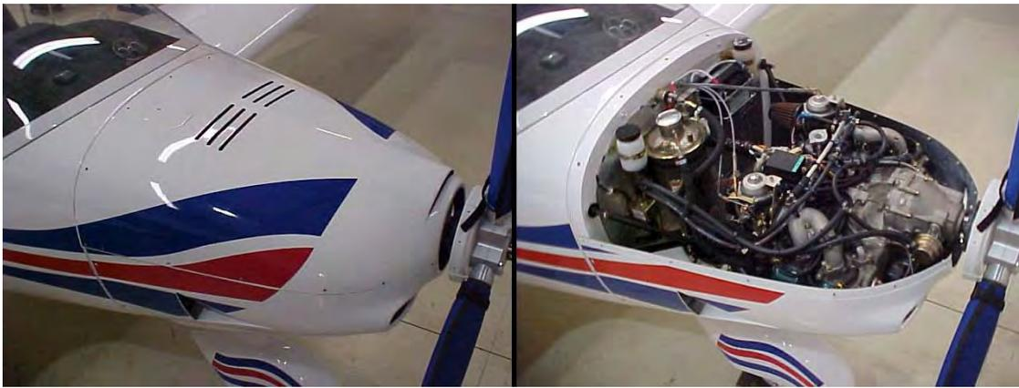
**Figure 6.1** Cowling removal
