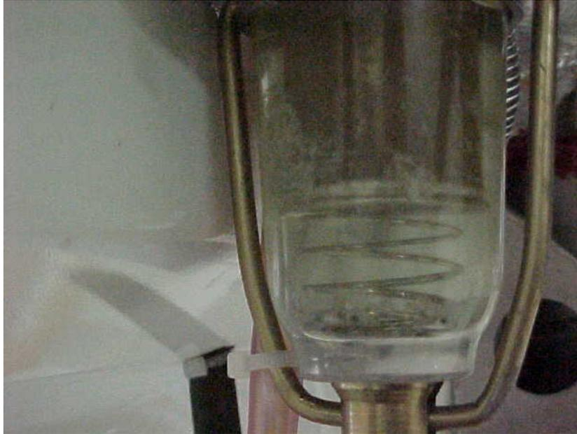
**Figure 7.62:** Fuel Filter Debris
