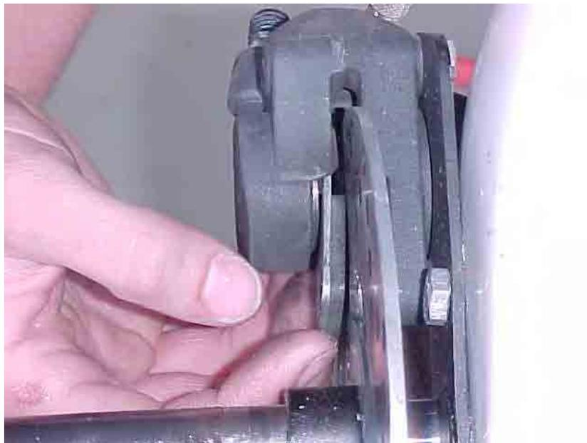
**Figure 7.5** Brake pad removal
