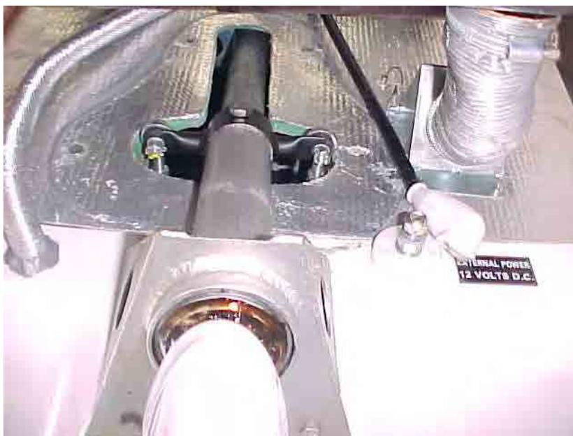
**Figure 7.42** Nose strut in place and bellcrank bolt installed
