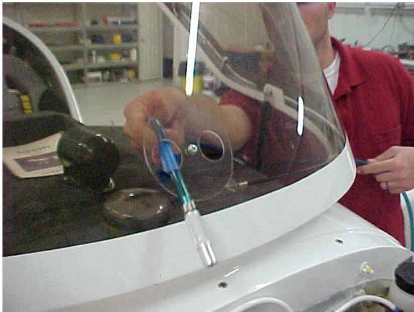
**Figure 7.46** Insert hoses through front vent window.
