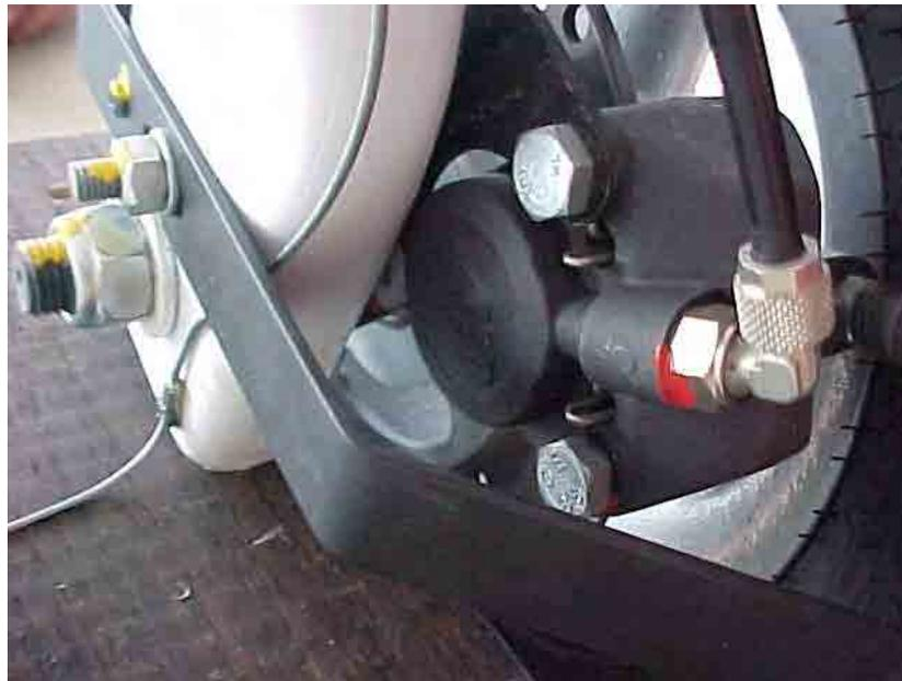
**Figure 7.9** Brake pad retaining pins installed
