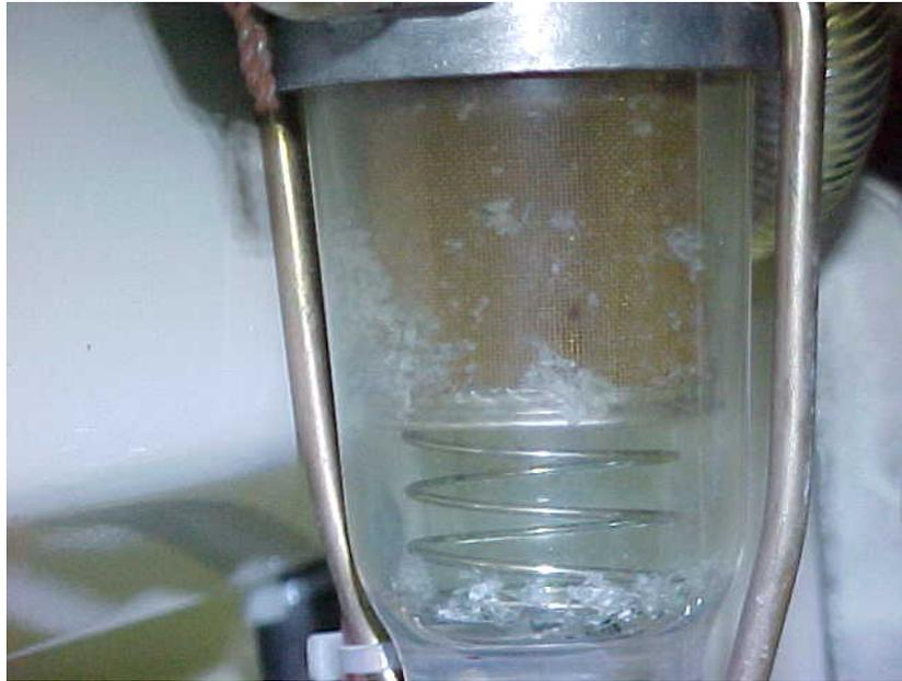
**Figure 7.64:** Fuel Filter Debris
