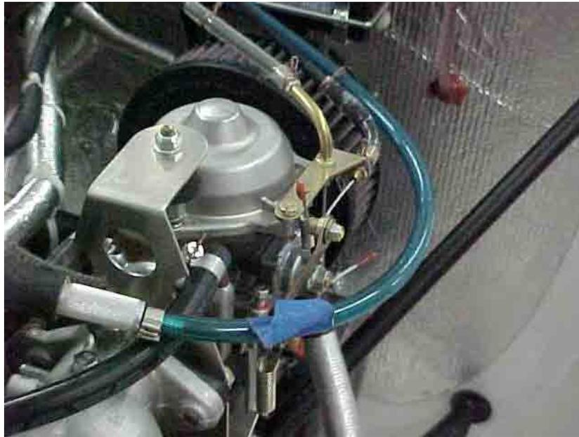
**Figure 7.55** Balance hose inserted through compensation tube.
