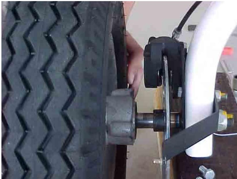
**Figure 7.20** Wheel and spacer in assembly
