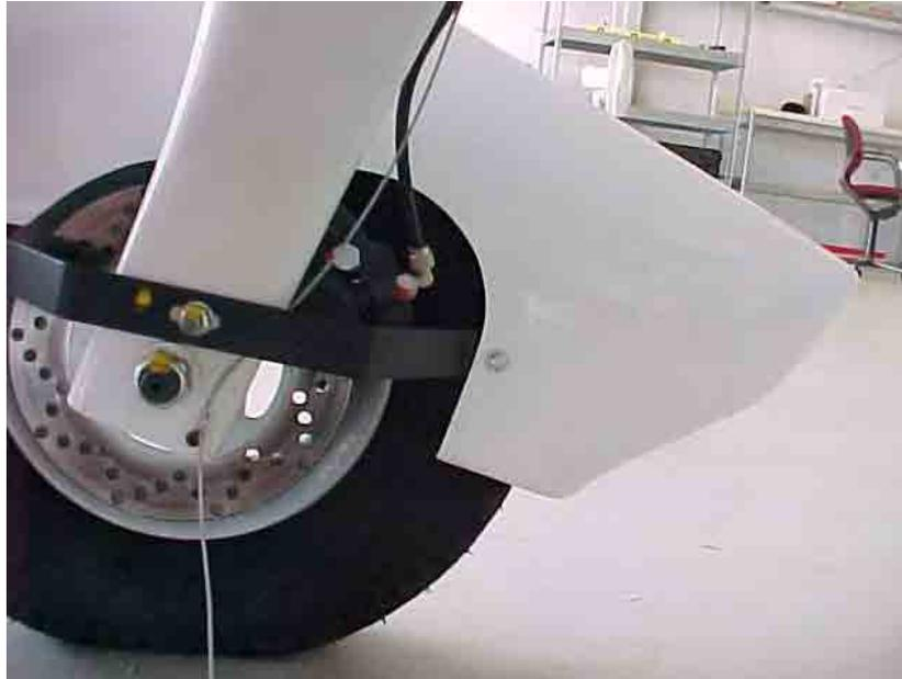
**Figure 7.11** Main wheel with brake caliper
