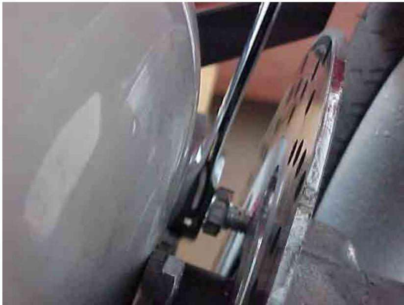
**Figure 7.16** Brake disk bolt removed from wheel assembly
