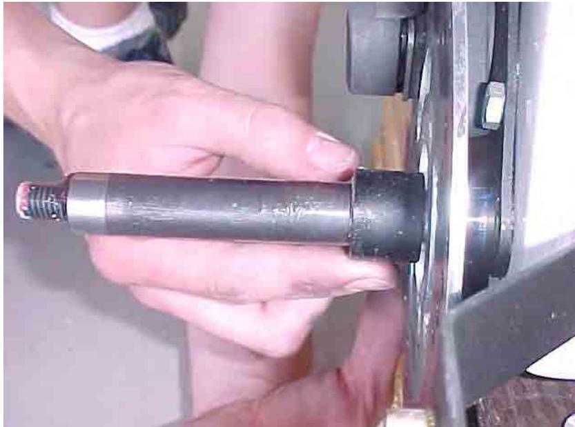
**Figure 7.19** Main wheel assembly spacer prior to wheel installation
