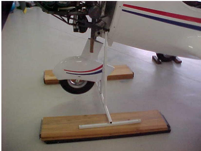
**Figure 7.28** Side view of nose support system
