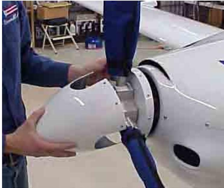
**Figure 6.2** Removal of the spinner
