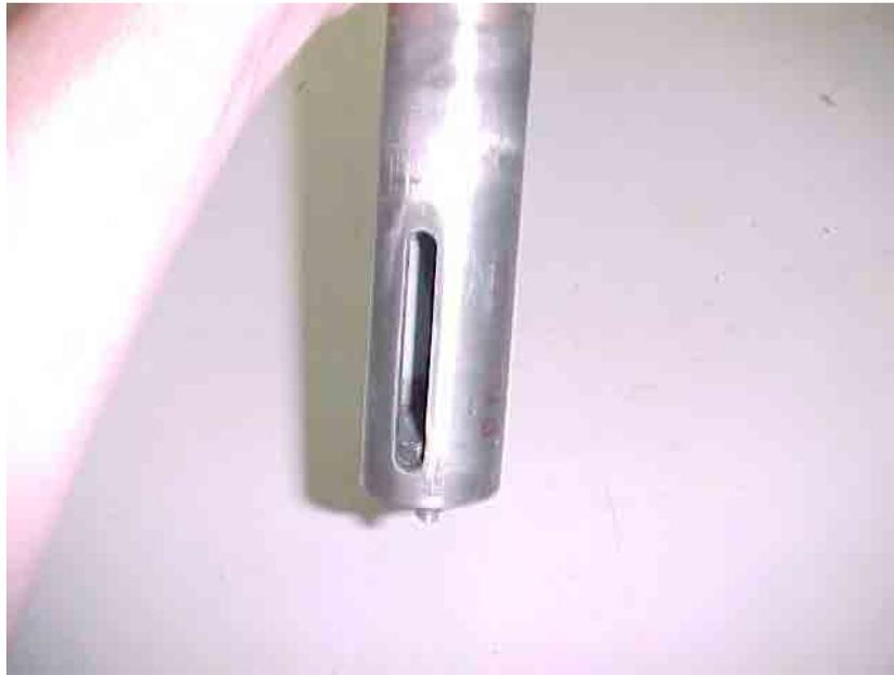
**Figure 7.40** Nose strut upper tube showing movement slot
