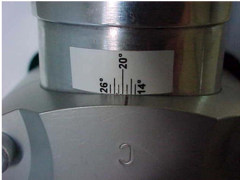
**Figure 6.7** Checking blade C pitch at 18 degrees.
