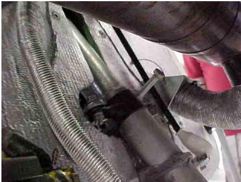
**Figure 7.33** Nose strut bellcrank bolt removed
