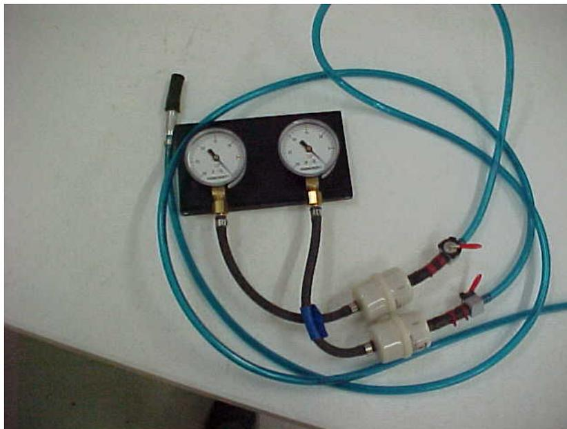
**Figure 7.44** Carb balance equipment with hoses, filters and check valves.
