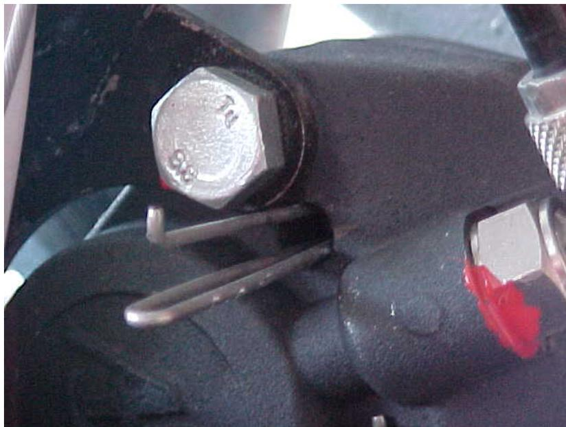
**Figure 7.3** Brake pad retaining pin removed
