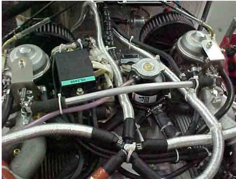
**Figure 7.47** Crossover compensation tube between carbs
