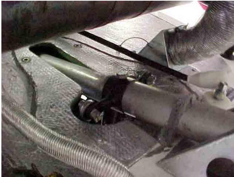
**Figure 7.32** Exposed nose strut bellcrank with bolt, engine side.
