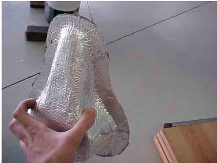
**Figure 7.31** Nose strut firewall cover removed.
