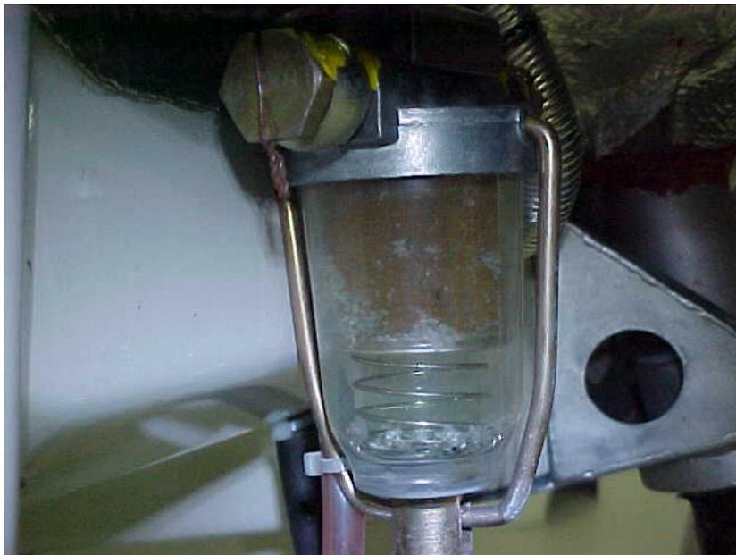
**Figure 7.63:** Fuel Filter Debris
