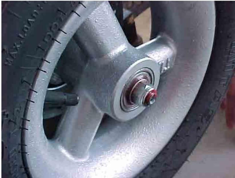
**Figure 7.23** Main wheel axle nut
