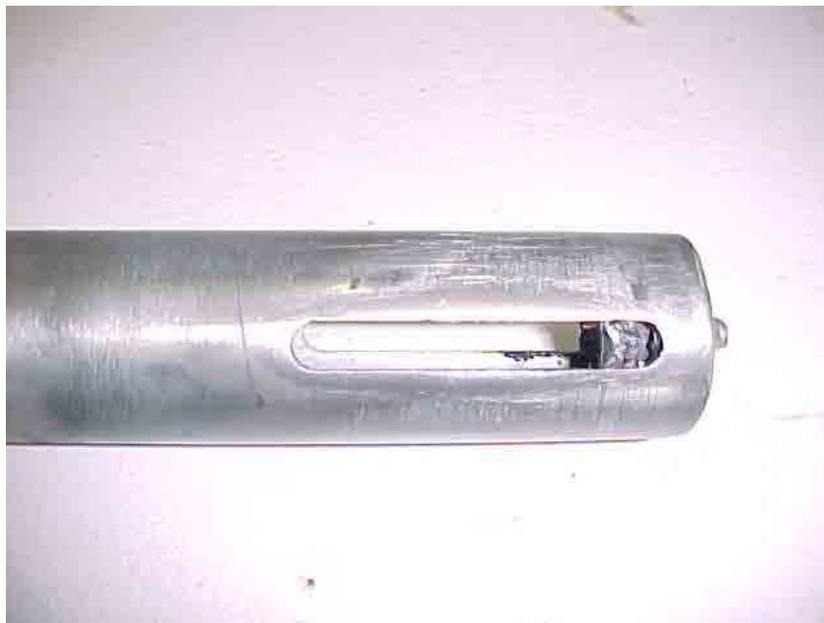
**Figure 7.41** Detail of movement slot to check for stress cracking
