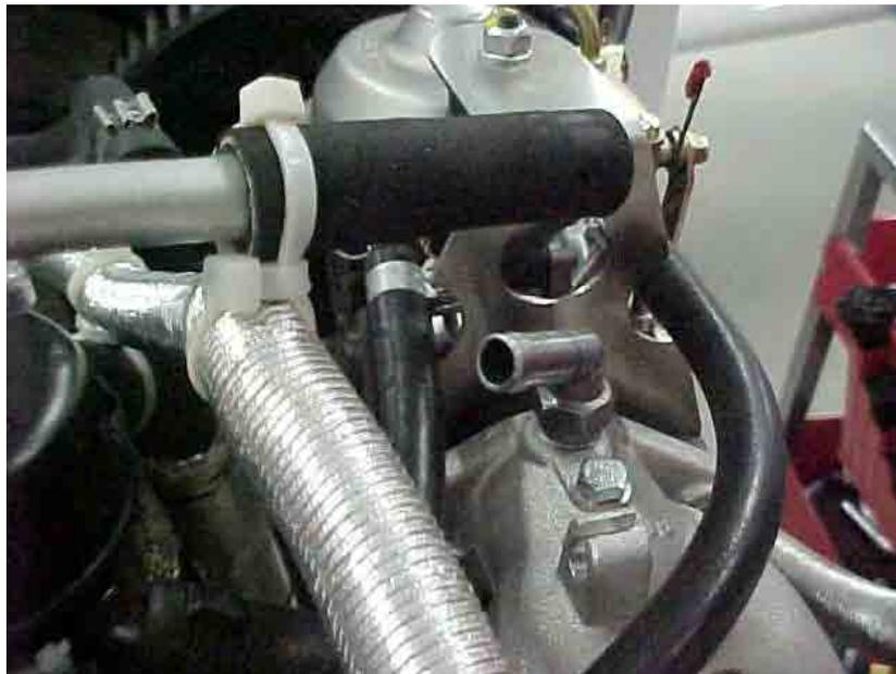
**Figure 7.52** Compensation tube hose removed from carb manifold
