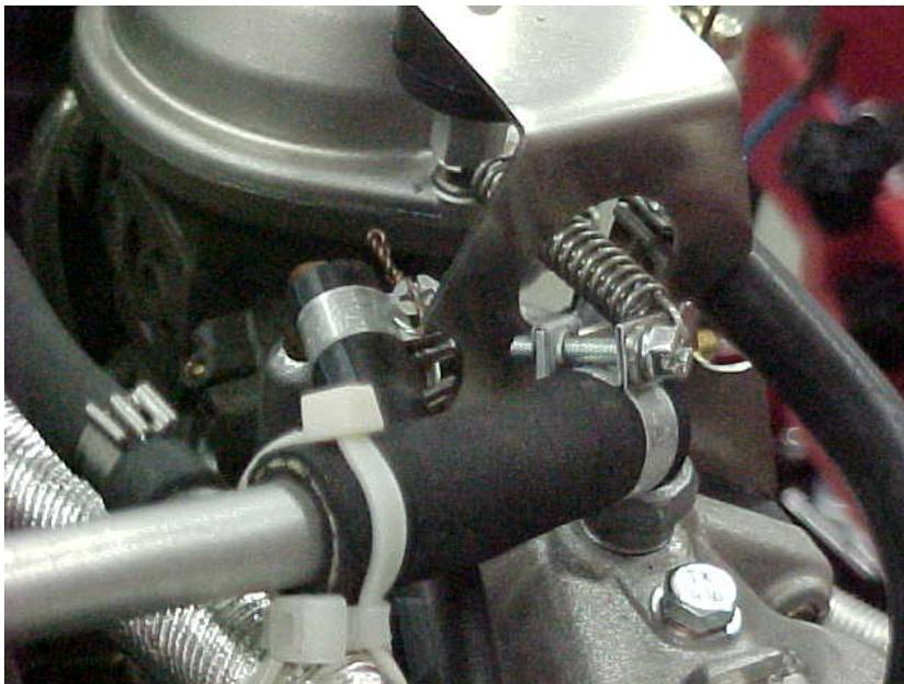
**Figure 7.48** Compensation tube attached to carb intake manifold
