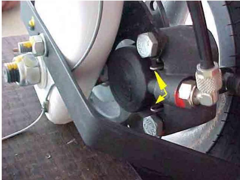
**Figure 7.2** Brake pad retaining pins
