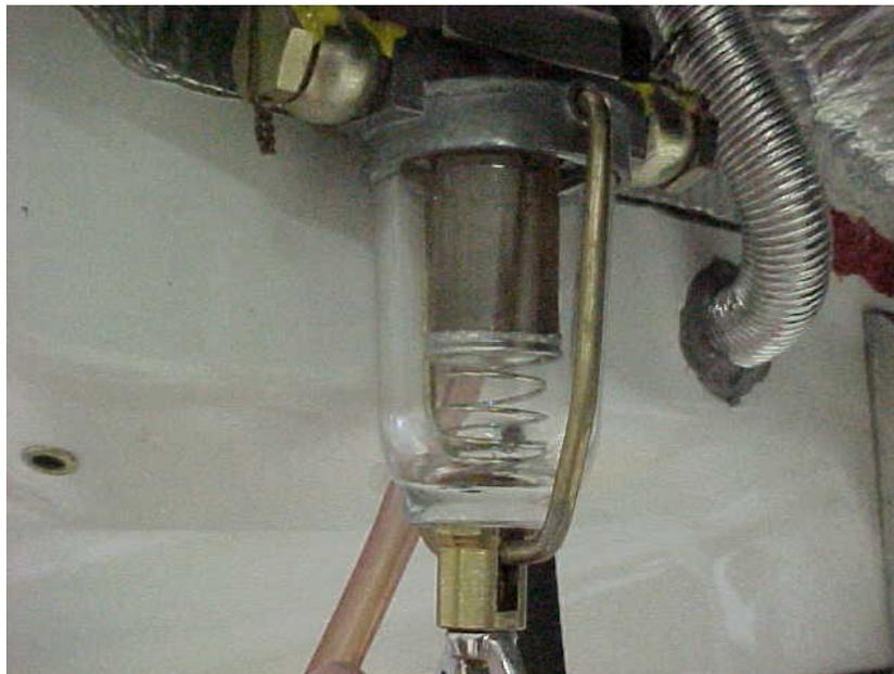
**Figure 7.68:** Fuel Filter supported by Spring
