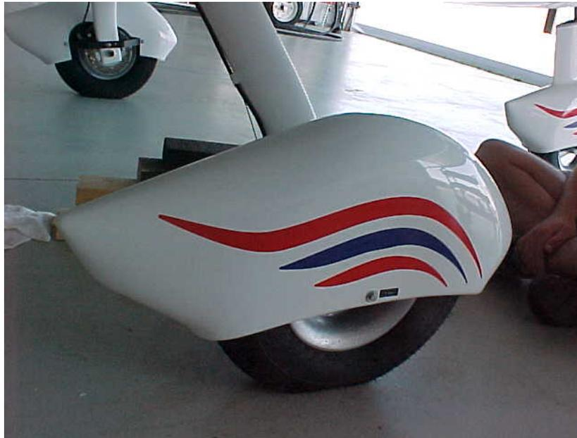
**Figure 7.25** Main wheel pant installed
