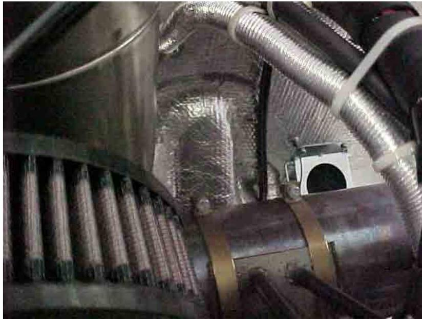
**Figure 7.30** Nose strut firewall cover from above
