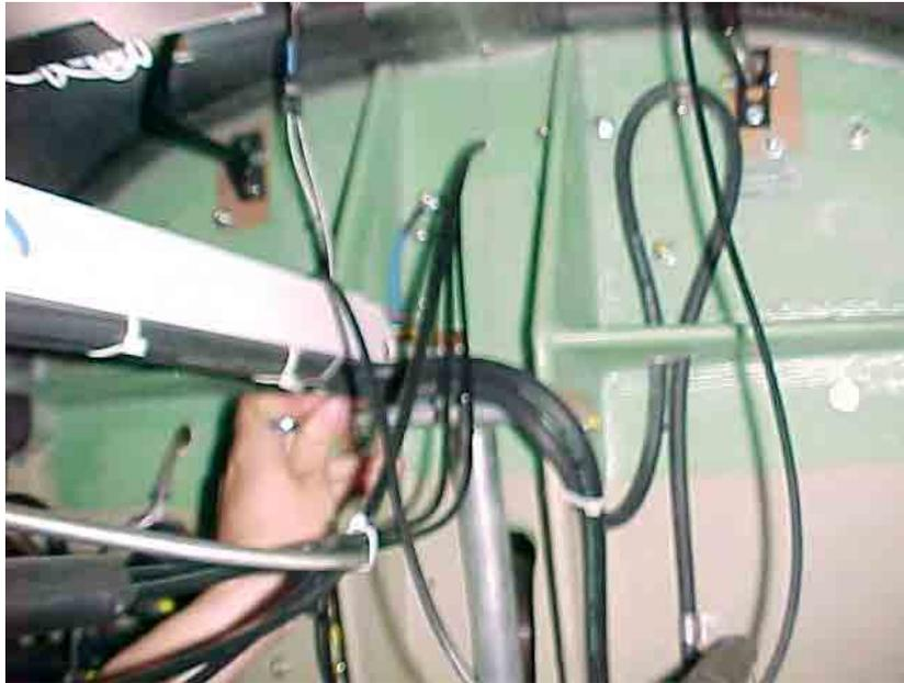
**Figure 7.34** Removal of the M8 nut on the top of the nose strut
