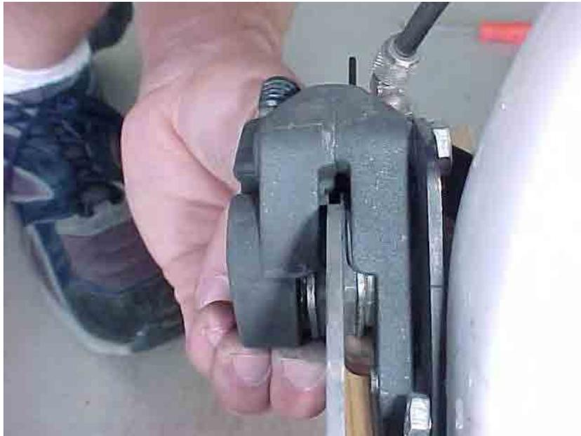
**Figure 7.8** Brake pad replacement
