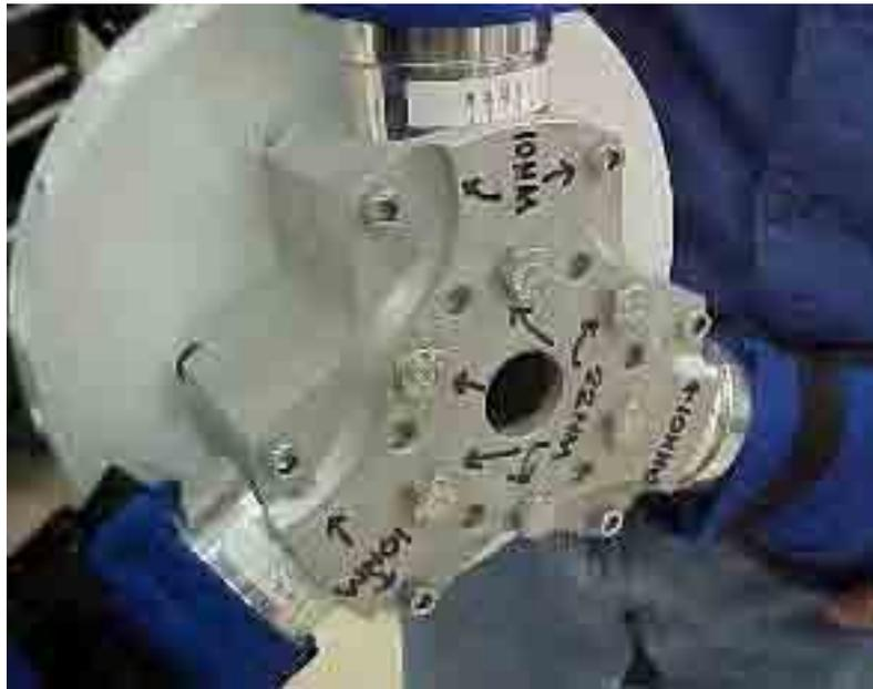
**Figure 6.6** Torque markings for each bolt
