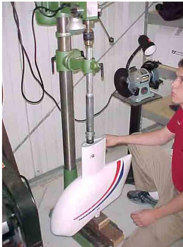
**Figure 7.38** Remove spring retaining bolt after spring is compressed.
